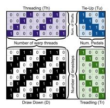
Figure 2: A weaving draft for a typical shaft loom. Drafts describe how warp yarns connect to shafts (threading), how shafts connect to pedals (tie-up) and how pedals are actuated (treadling) to create the weaving pattern (draw down).
