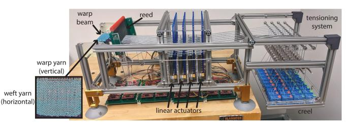
Figure 1: Semi-automated Pattern Executing Educational Robotic Loom (SPEERLoom): An open-source robotic Jacquard loom kit for use in interdisciplinary collegiate classrooms
