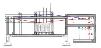
Figure 5: Different warp yarn positions in SPEERLoom. Each heddle can be either raised or lowered, with the same amount of tension pulled on the warp yarn in either position. Yarns (blue and red) pass through the tensioning system and over the guiding rods before going through the heddles.
