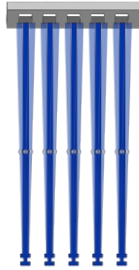
Figure 11: An example of physicality, where the alignment of heddles with the guide requires manipulating multiple objects simultaneously to keep them aligned as the guide is put over the top. This can provide opportunities for coordination, cooperation, and communication.
