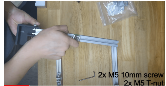
Figure 12: A screenshot from the RoboLoom assembly instructions showing a step of assembly. The written text document for assembly lists this instruction as “Put the holders onto the bottom square pieces... Put a screw through the holes and each side of the foot holder and screw on a t-nut to each screw. Slide the 8020 into the holder.”
