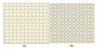
**Figure 4** *Fabric planning for producing unit circles*
