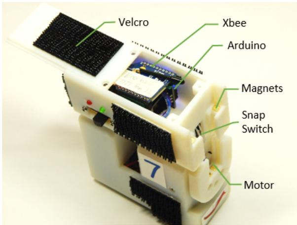
Figure 5. Electronics in the Joint Modules
