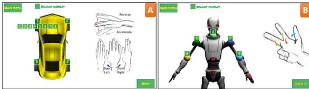
Figure 3. Tablet Interface for selecting position of the joint module (a) four wheel vehicle (b) puppet
