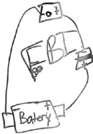
Fig. 5 Omarosa's FBI T-shirt circuit design page from her journal, illustrating where the battery placement, LED and switch were to be arranged around the "FBI" design on her T-shirt
