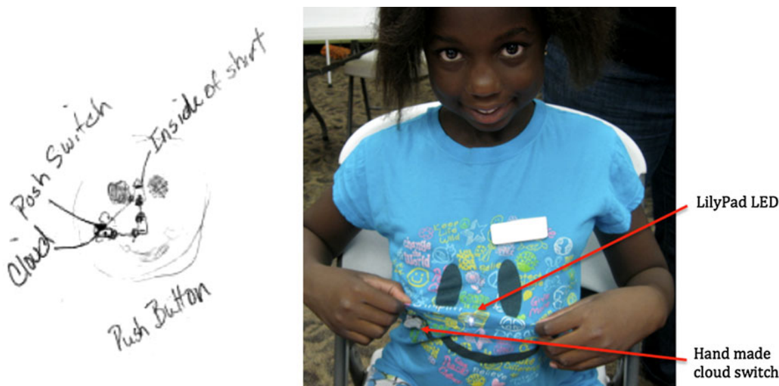
Fig. 4 T-shirt drawing and finished product with working circuit, handmade cloud switch and hidden battery holder inside the shirt
