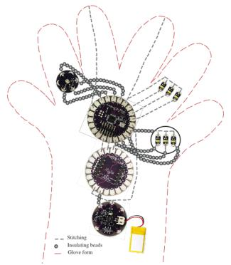
Figure 2. Layout of the ForagerBee Glove
